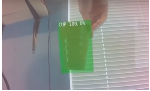
Fig. 8. A red plastic cup being detected by the camera on Trash-E using the object detection model.
